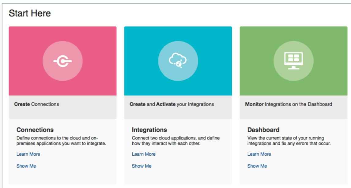
Figure 6 – As you sign into Oracle Integration Cloud Service, a “Start Here” screen leads you through the simple steps of “Connections”, “Integrations”, and “Dashboard” to connect to the applications, transform data between the applications, and monitor flows between applications.
